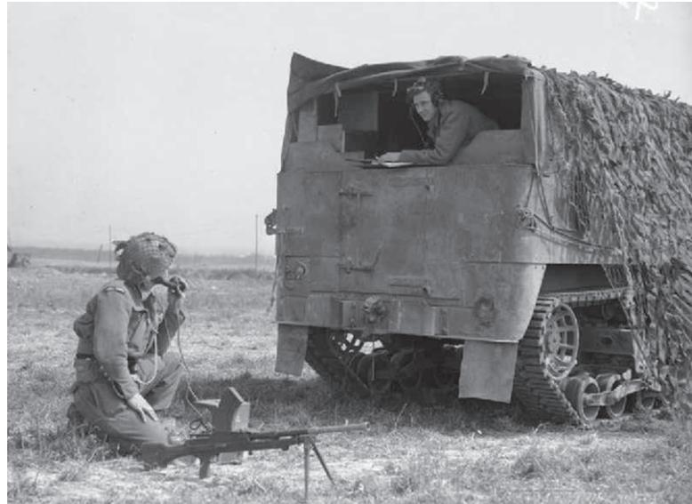
(Above) M14 half-track in France used by a British Royal Navy Forward Observation Bombardment unit. This is probably a “Truck 15 cwt. half-tracked Command” judging by the radio sets at the left rear, even though these “should” be fitted in the middle rather than at the rear. (Source: [IWM A 24353](#))
